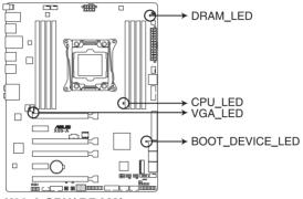
X99-A CPU/ DRAM/ BOOT DEVICE/ VGA LED
